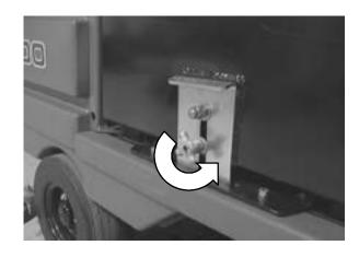
10. Raise the battery latch plate up out of the securing slot.
